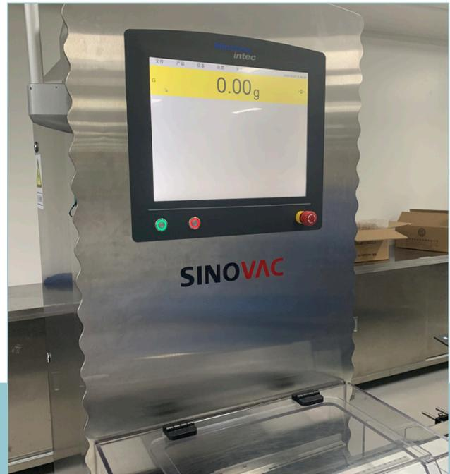
For Sinovac the checkweigher Synus ensures reliable rejection of incomplete products at a throughput rate of 260 pieces per minute
