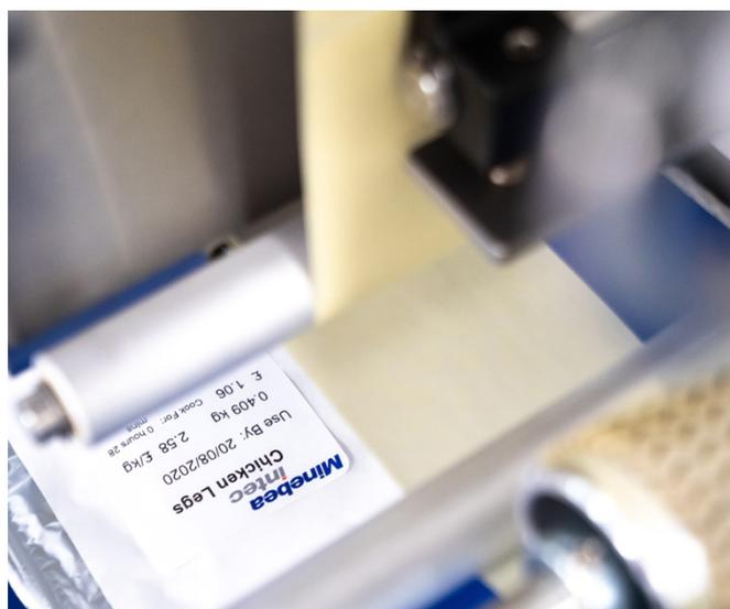
The WPL-A convinces with high-speed printing of up to 125 labels per minute, made possible using advanced print compression technologies.
