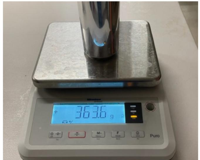
Puro® SmallFlat scale with yellow indicator showing an under-fill
