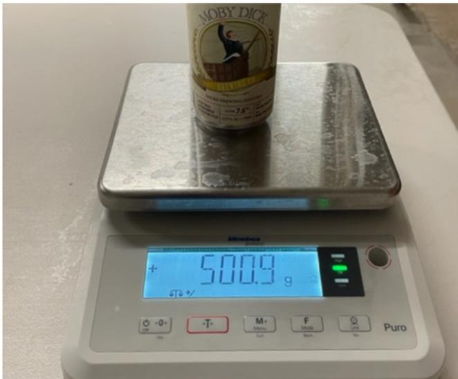
Puro® SmallFlat scale with green indicator showing the contents is in tolerance
