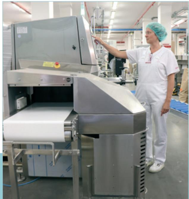
The X-ray inspection system Dymond is permanently installed as a critical control point at the end of Anona's production line
