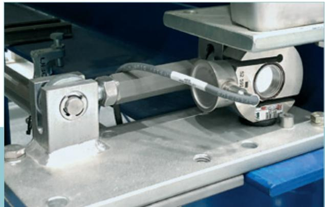
The S-type compression load cells under the additive container tanks provide highly precise measurement results
